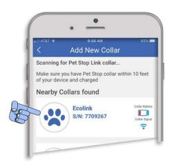
When you select the collar you wish to pair, you will be asked to set a 4-digit **PIN** (we recommend using the last 4 digits of the **serial number**). Once you've entered your **PIN** the **Pet Detail** screen will open. Within the **Pet Detail** (see pg. 10) screen, you can now press **Connect** to activate the collar for use. Once connected, the **Connect** button changes to **Disconnect**, which you can press when you want to disconnect or switch collars.
